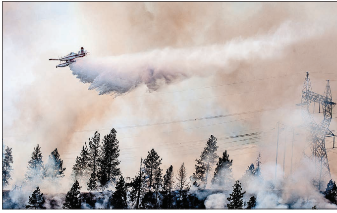
A Fire Boss single-engine air tanker makes a drop. Idaho Department of Lands via Capital Press
