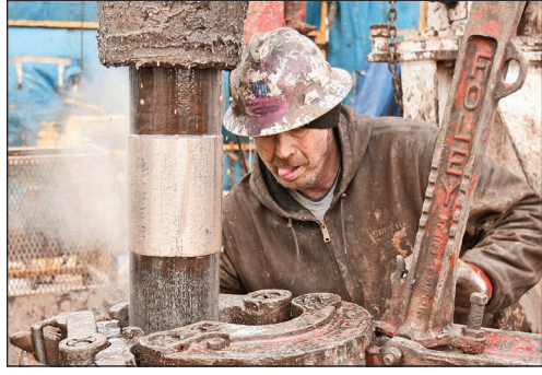
Deckhands on a Sandridge Energy oil rig change out a drill pipe in a fracking operation on the Oklahoma border in Harper County, Kansas.
