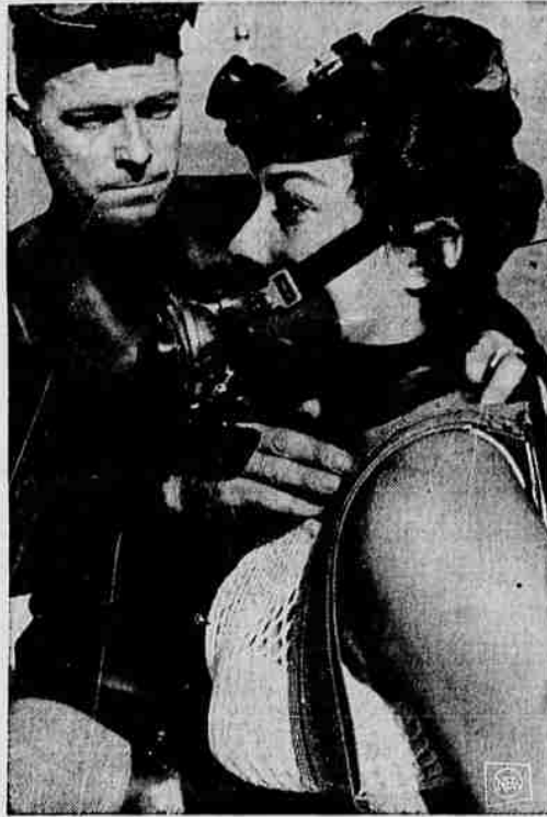
WATER INTER-COM —This one-way underwater communication device will soon have Scuba divers looking over their shoulders for that "voice." This Bendix Corp. electronic system can be heard by divers within an underwater range of 100 yards with the human ear as the only receiver.
