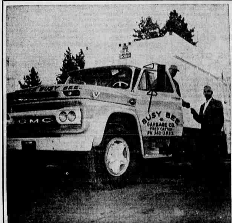
Morley Madden is shown presenting the keys to Fred Carter, of the Busy Bee Garbage Co., for a 1964 GMC 2 1/2-ton Truck. Some of the outstanding features include 16 yard Heil Collectomatic Mark II box with a hydraulic packer and a 2 yard capacity hopper only 29" high for clean, quick garbage collection. Mr. Carter has leased this truck from Central Oregon Auto Lease, Inc. who repeat: "We are prepared to lease anything that rolls on wheels!" If you're thinking of leasing, drop out and see Morley Madden at Murray & Holt Motors, Inc., 181 E. Franklin for more information. Adv.
