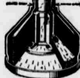
Cross-section of new bowl, showing new method of distributing milk between the discs.
