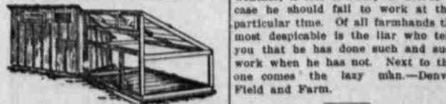
stringers, and the frame is held on the floor by blocks at each corner. Lumber required will be: 12 pieces, 2 in. x 4 in., 16 ft. long for frame; 4 pieces, 1 in. x 12 in., 16 ft. long for floor; 13 pieces, 1 in. x 2 in., 16 ft. long for roof and ends; 10 battens, 16 ft. long for sealing crack between boards. Total cost about \$12.50.
