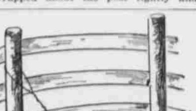
HOW TO BRACE A FENCE POST.
