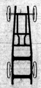
frame - not on the body sills. The body and the frame form a rigid unit that successfully resists the rack of the road. Studebaker bodies are built in Studebaker
