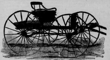
It is light, strong, easy riding, and well made, having three elliptic springs underneath the y (these springs are made especially for this wagon and will carry 500 s, with ease), double ar, steel axles, the best steel tire, leather dash, and a solid bear ed bottom. It has a box for the seat for small packages, and a wire guard around the seak for holding larger packages. Send for catalogue and prices. Manufactured by GAP DINER & CROSS.
