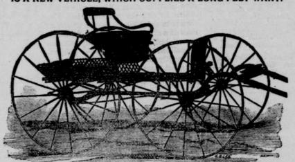
It is light, strong, easy riding, and well made, having three elliptic springs underneath the body (these springs are made especially for this wagon and will carry 500 lbs, with ease), double collar, steel axles, the best steel tire, leather dash, and a solid beaded bottom. It has a box under the seat for small packages, and a wire guard around the back for holding larger packages. Manufactured by GARDINER & CROSS.
