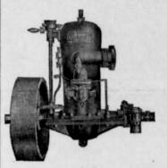
represent a distinct step in advance in marine engina construction. No outside water pipes, not an ounce of superfluous weight, all bearings adjustable to take up wear.
