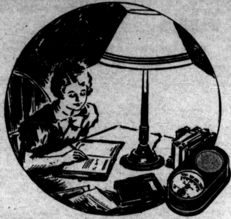
The Light Meter, an instrument for measuring light, reads 20-30 footcandles under an I. E. S. Study lamp.
