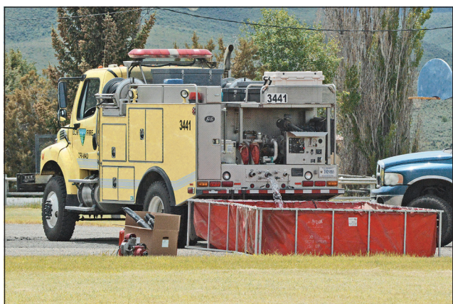
A BLM 800 gallon all-terrain fire truck fills a portable tank, known as a “pumpkin,” on June 9, 2022, at Burnt River School in Unity.
