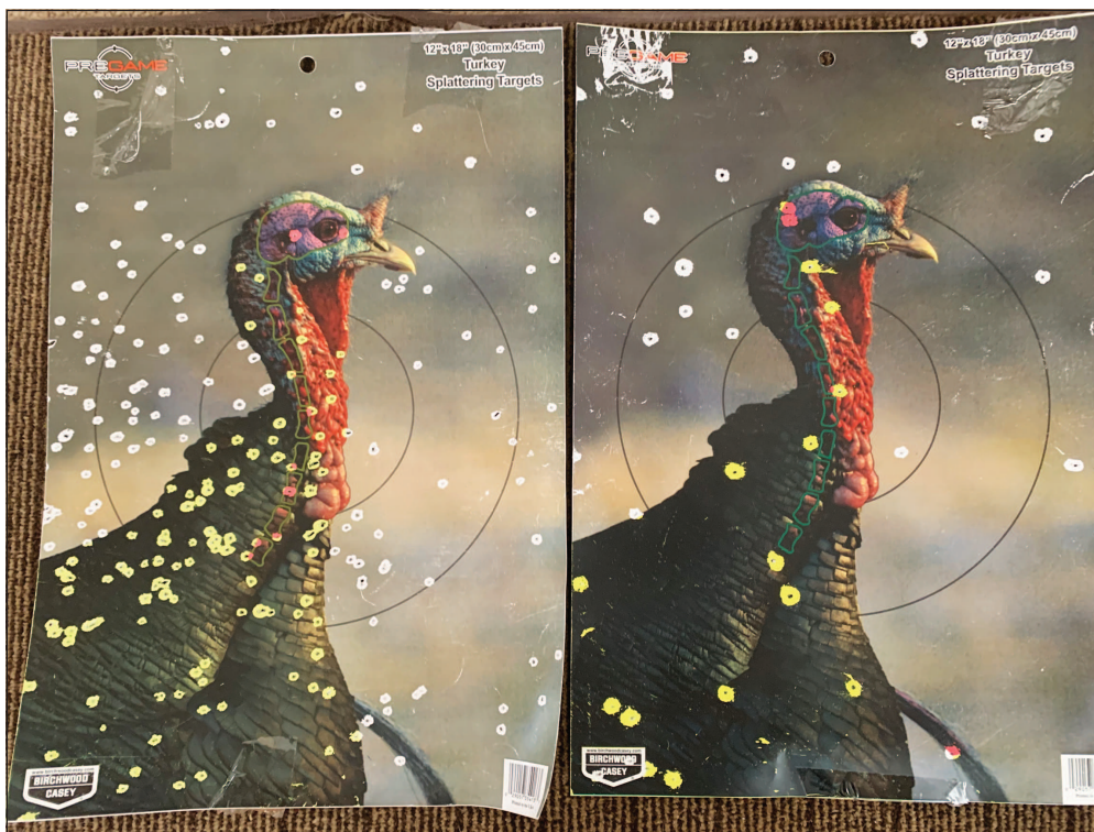
As these targets show, the shot pattern can vary substantially with different shells
