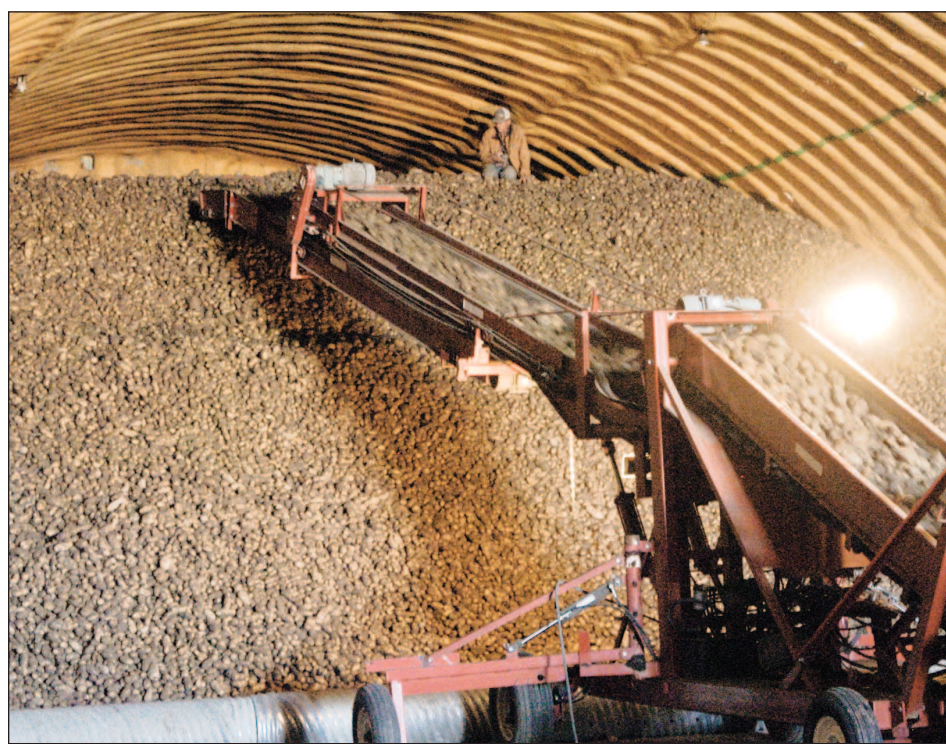
Robert Adams perches atop the pile to guide the conveyor's distribution of potatoes evenly from front to back inside the cellar, which can hold 3,000 tons of spuds.
