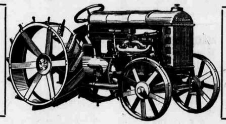
All gears run in a bath of oil so simple any one can handle them.
