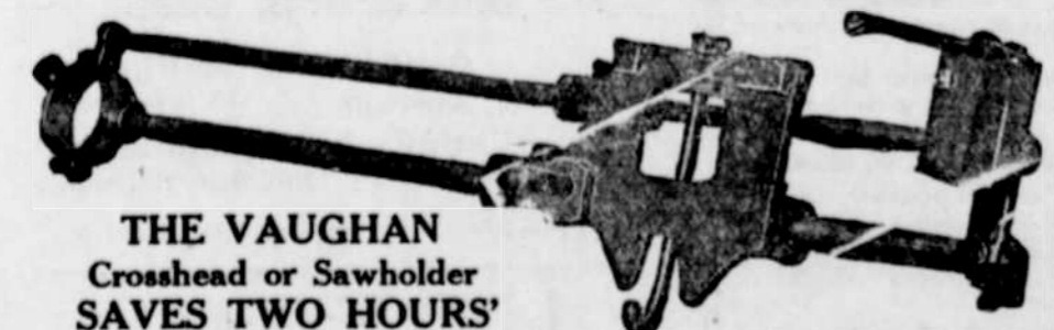
For cutting cordwood, clearing land or sawing logs. Our machine naturally fits itself to the different positions while sawing without any adjustment.
