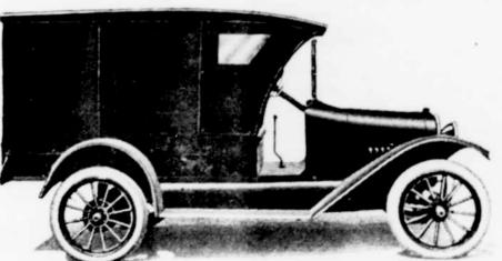
Top complete, with rolled side and back curtains made of heavy oiled duck.
