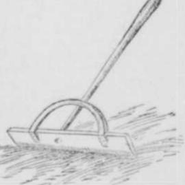
and lawns. The board can be of considerable length, sharp at one edge, with a bit of flat iron riveted to the edge, the used-up blade of an old wood-saw being excellent for this purpose. The handle is braced firmly by a half-circle of iron which a blacksmith can fit in place in a few moments. With such an implement the work of leveling and grading can be done quickly and easily. It should have a piece in any garden kit.
