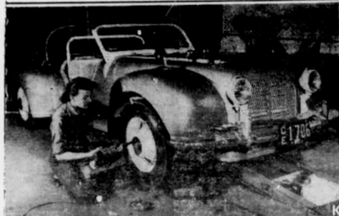
Grace Curry, Miss Autorama of 1956, checks her "Doodlebug" which she races Sundays down the drag strip at Woodbine, N. J. Capable of hitting 120 miles per hour, the car is a custom-made model, built by Grace herself. Here she checks over the wheel lugs for proper tightness with an Ingersoll-Rand Torque Control Impactool. First and only electric torque control wrench in the world with optional Torsion Bar Torque Control, the tool automatically spins down nuts to a preset torque and then shuts itself off. If the nut is tight enough, the tool will not operate. A hybrid of many parts, the "Doodlebug" has a Mercury '48 engine, Offenhauser heads and a 2-pot manifold. It is built on a '40 Ford frame, and runs on '35 Ford wheels. The hand-formed aluminum body has Pontiac taillights set in reversed Studebaker truck fenders.
