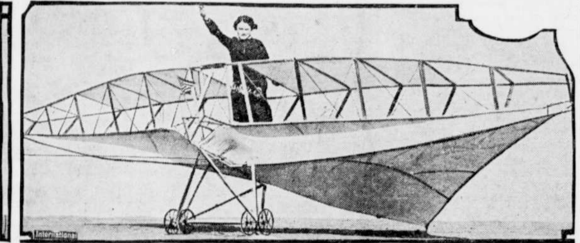
Shown to the public for the first time, after more than 200 trial "flights," this huge passenger-carrying kite is being studied by aero experts at Los Angeles. Invented by George A. Argabrite, who has flown kites since school days, it has been tested and so far has carried 180 pounds aloft. The photo shows Mrs. Argabrite in the kite.
