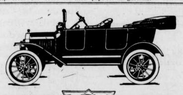
Especially resistant to shock, strain and vibration, toe Ford is the sturdiest, most durable car in the world. Vanadium steel, heat-treated by the Ford process, accounts for the strength and light weight of the Ford car. Strong, light, simple and efficient, the Ford gives service and satisfaction to more than 700,000 owners every day, at an average cost of two cents a mile for operation and maintenance.
