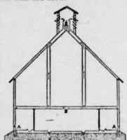
Another arrangement of flues which is quite effective in securing ventilation. The opening in the center of B may be provided with a shutter to prevent too rapid movement of air. Separate outlets may be provided or he single cupola as shown.
