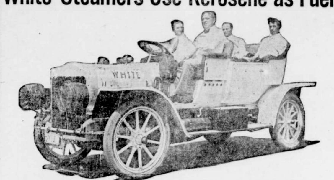
THE WHITE STEAMER WHICH MADE A SUCCESSFUL PUBLIC DEMONSTRATION OF KEROSENE AS FUEL ON THE RECENT 2655-MILE GLIDDEN TOUR.
