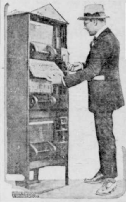
An inventor in Los Angeles has just completed this machine, whereby it is possible to drop your coin in a box, turn a handle and secure your favorite paper.
