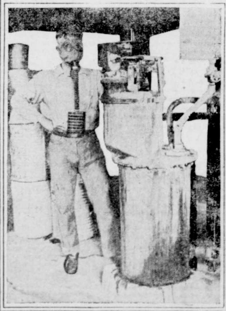
Picture in one of the seven poison plants on the Texas border where trains from Mexico are fumigated with deadly cyanogen gas to kill the destructive pink boll weevil whose home is Mexico.
