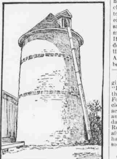
A CEMENT BLOCK SILO.
