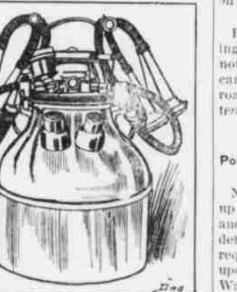
LATEST TYPE OF MACHINE MILKED. apparatus, tubes, receiving can, milk cups, etc., can be fixed at one spot. This makes it unnecessary to shift the appliances so frequently.
