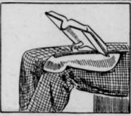
sons who are near or far sighted it is only necessary to slide the support back and forth between the keepers until the focusing point is reached. As the support can be made of aluminum, adding little to the weight of the book, and as it is placed on a member of the body which can support its weight directly on the floor, the book can be maintained in position much longer than if held in the hands.
