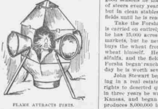
FLAME ATTRACTS PESTS. trap, the invention of a Kentuckian, will receive a share of attention and serve its purpose in many a field. The inventor takes advantage of the well-known propensity of insects to fly toward a light, the flame in this instance being mounted within a metallic casing, to which entrance is gained through four funnels pointing in different directions. Once within the hood, the insect soon falls to the reservoir beneath, wherein a quantity of insecticide has been placed to complete the destruction of those which escape the actual contact with the flame. Mention is also made of the fumes rising from the liquid and impregnating the atmosphere around the flame to overcome the insects and cause them to fall into the liquid.
