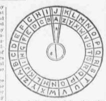
letter of the keyword in the outer wheel. Take out at once for the whole In the clober wheel the letters of message the clober letter of the liner the keyword and those of the true mes- wheel corresponding to the true letters sage are taken from the outer ring, on the outer which appear above the letters of the cipher message being the first letter of the keyword whenevar it occurs.
