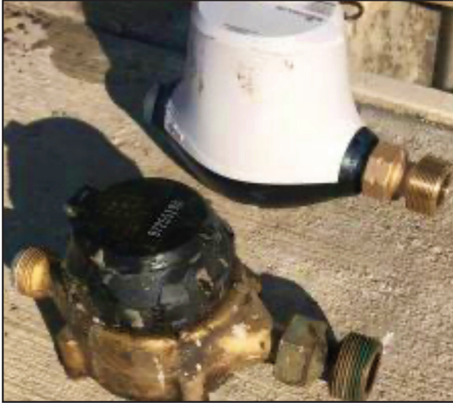
The city's mechanical water meters (left) have been completely replaced by new, automated meters.
