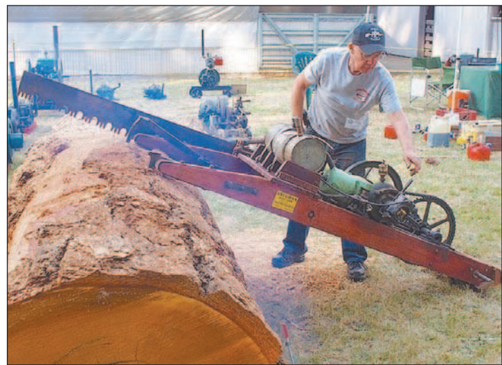
photo by Bruce Kelsch Bill Gaywell demonstrates his Vaughan two-cycle gas powered drag saw from the 1920s.
