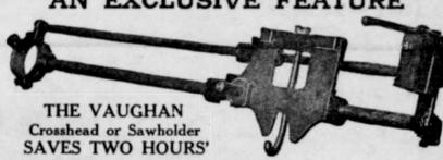
time a day. In a jiffy the saw blade is put in or taken out of the holder and the operator loses no time fussing with nuts or adjusting the holder. This feature is covered by patent and is only on the VAUGHAN. The holder bolt engages under side of blade and holds it firmly up against lugs on top and face of sawplate crosshead. Write for further information, special terms and prices.
