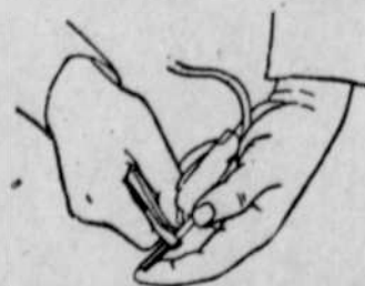
Crimping the Cap to the Fuse.
