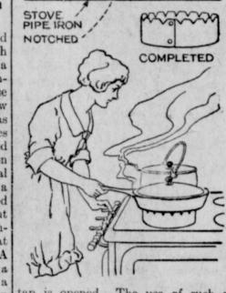
ring concentrates the heat under the vessel and consequently reduces the onsumption of gas.
