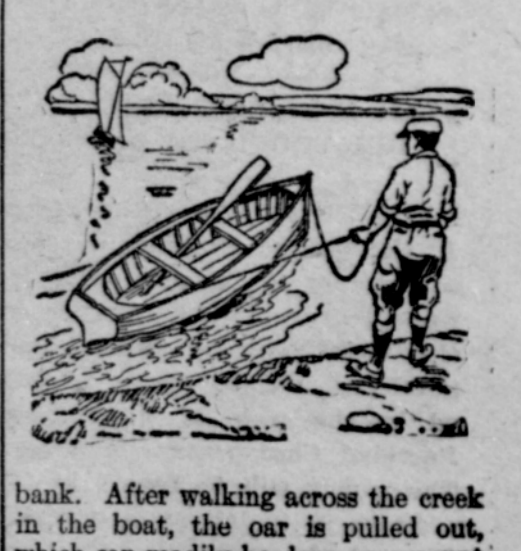
Towing Small Boats: When the stream is flowing so fast or the wind blowing so hard that it is difficult to make headway by rowing, the simple stunt shown in the drawing offers an easy way of towing the boat along the bank or shore.
