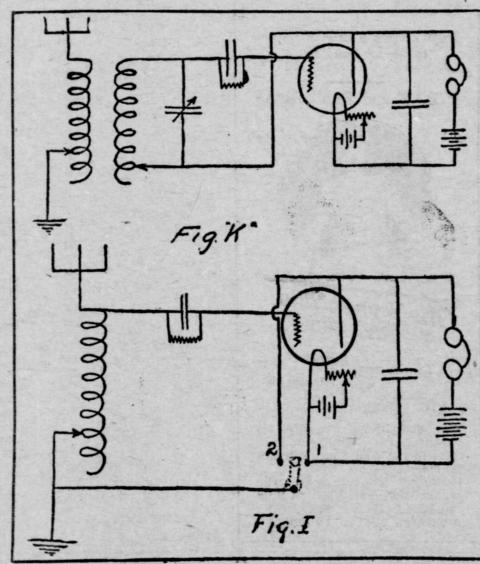
ty of the large new poultry build- tive circuit. When the two-point switch is on contact No. 1, the set is non-regenerative. Turning the switch to point No. 2 makes the set regeneradreds of extra coops, which have tive. The circuit arrangement for rebeen placed in every available inch generative is known as the ultra audion circuit
