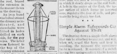
himney extension and to the stovebolts, and were spread apart by means of a steel hoop, which was held in position by wrapping each guy wire around it once. This bracing made the extension so strong that it has with stood the heaviest gales.
