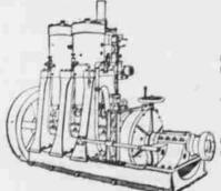
Using gasoline or cheap distillate off Engines connected direct with propeller shaft, and no noisy, easily broken bevel gears used in reverse motion. New spark device: no internal spring electrodes to burn out.
