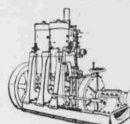
Using gasoline or cheap distillate oil. Engines connected direct with propeller shaft, and no noisy, easily broken bevel gears used in reverse motion. New spark device; no internal spring electrodes to burn out.
