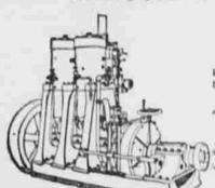
Using gasoline or cheap distillate off. Engines connected direct with propelier shaft, and no notsy, easily broken bevel gears used in reverse motion. New spark device; no internal spring stectrodes to burn out.
