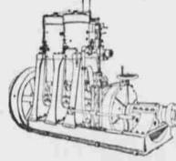
Using gasoline or cheap distillate oil. Engines connected direct with probevel gears used in reverse motion New spark device; no internal spring referedes to burn out.
