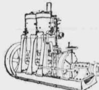
Engines connected direct with propetter shaft, and no noisy, easily broken bevel gears used in reverse motion. New spark device; no internal spring
