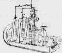
Engines connected direct with probevel years used in reverse motion.
