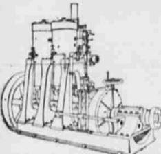
Using gasoline or cheap distillate oil. Engines connected direct with propeller shaft, and no noisy, easily broken bevel gears used in reverse motion.
