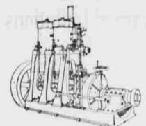
Using gasoline or cheap distillate oil. meet Engines connected direct with propeller shaft, and no noisy, easily broken beyel gears used in reverse motion. New spark device; no internal spring electrodes to burn out.
