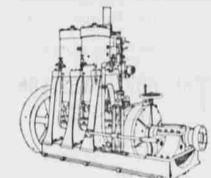
Using gasoline or cheap distillate oil. bevel gears used in reverse motion.
