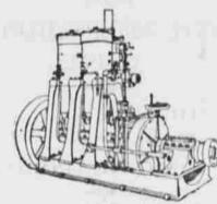
Using gasoline or cheap distillate oil. Engines connected direct with propeller shaft, and no noisy, easily broken bevel gears used in reverse motion. New spark device; no internal spring if it becomes a law. electrodes to burn out.
