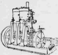
Using gasoline or cheap distillate off. Engines connected direct with propeller shaft, and no noisy, easily broken bevel gears used in reverse motion New spark device; no internal spring
